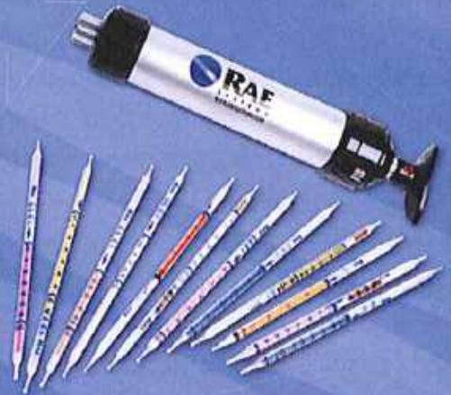
RAE Systems colorimetric gas detection tubes enable quick, on-the-spot measurement of a wide range of toxic and combustible gases and vapors. RAE Systems tubes are easy to read, and provide a sharp, clear color change directly corresponding to the concentration of gas present. RAE Systems tubes are compatible with the RAE Systems piston hand pump, a reliable way to draw samples of an exact volume required for the most accurate measurements.
